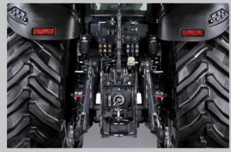
12,000 kg lifting capacity, 210 l/min pump output, three PTO speeds: designed to master any implement.
