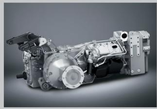
Optimum efficiency: continuously variable TTV transmission for a top speed of up to 60 km/h with a lower engine speed.
