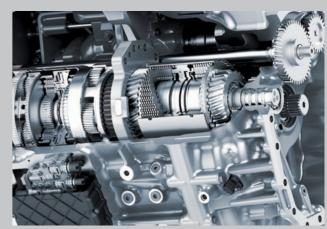
Continuously variable TTV transmission with a speed range from 0.2 to 60 km/h at reduced engine speed. Perfect precision.
