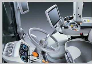
MaxiVision 2 cab with newly designed armrest and 8" or 12" iMonitor. Maximum comfort for maximum driving capacity.
